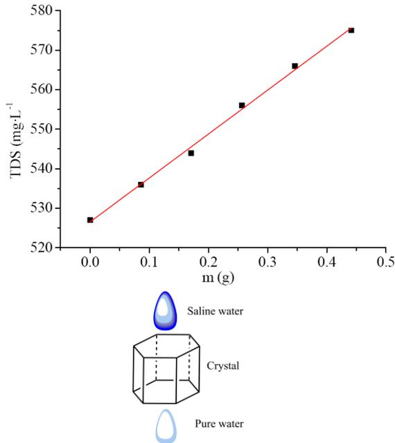
**Figure 2.** The static desalination results of dehydrated  $\{La(H_2O)_4[La(1,3-pdta)(H_2O)]_3\}_n \cdot 12nH_2O$  (**1b**).
