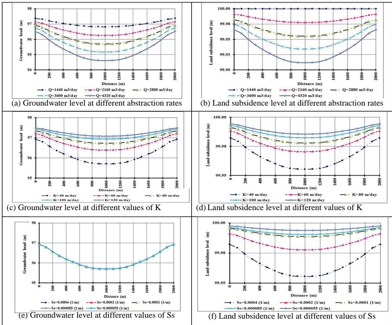
Figure 3. Results of groundwater level and land subsidence level for different scenarios
