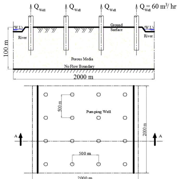
Figure 1. Plan and vertical cross section of the hypothetical case study
